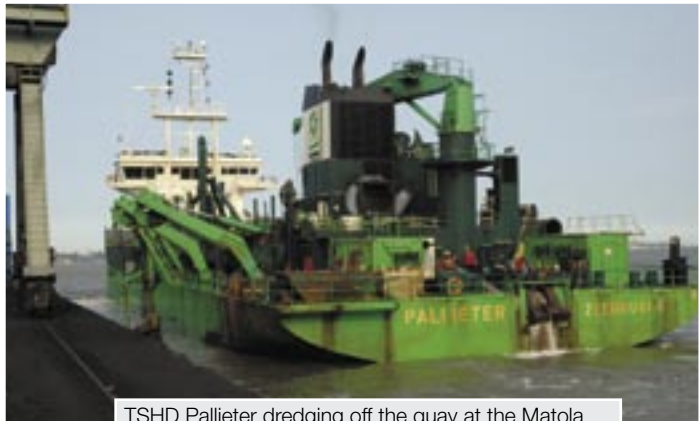
TSHD Pallieter dredging off the quay at the Matola Coal Terminal in the port of Maputo recently. The dredging project was completed in January 2011. A number of quays were dredged back to their original design depths.
