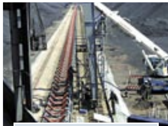
Top: The Stackler Reclaimer 2 reclaim chute at ground level for transfer onto yard conveyor.
