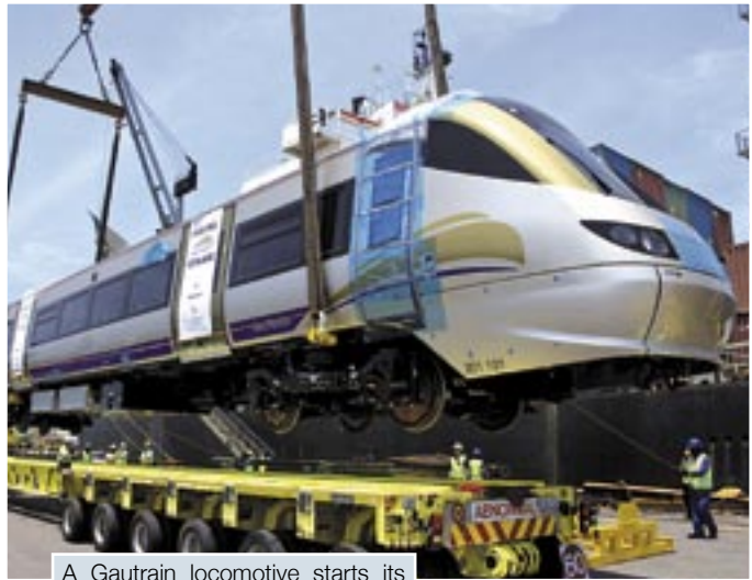
A Gautrain locomotive starts its first journey in South Africa: 800 km by road on a Vanguard trailer.
